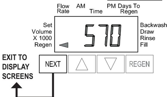
**Step 1D** - Press ▲ and ▼ simultaneously for 5 seconds and release. Then press ▲ and ▼ simultaneously for 2 seconds and release. If screen in Step 2D does not appear the lock on the valve is activated. To unlock press ▼, NEXT, REGEN, ▲ in sequence, then press ▲ and ▼ simultaneously for 5 seconds and release. Then press ▲ and ▼ simultaneously for 2 seconds and release.
