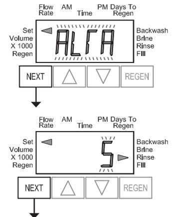
Selecting the Control Valve to act as a single valve twin alternator
